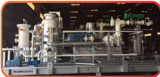
Process Gas Compression System
